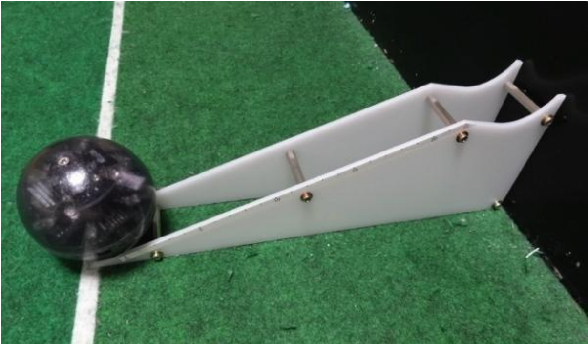
Fig. 1. Kicker Power Measuring Device
