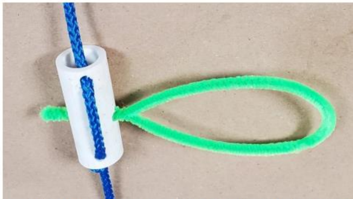
The algal marine growth inserted into a 3/16-inch hole in a short (variable) length of PVC pipe attached to the rope of a floating wind turbine.
