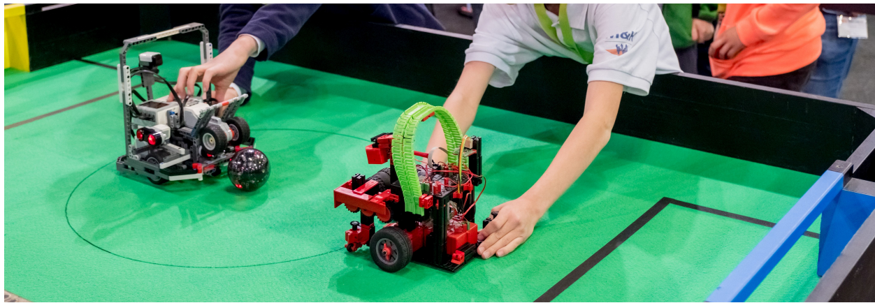
Figure 1 Two teams with one LWL robot each will compete using an IR ball on RCJ Soccer fields without the out-area. There is no need for using camera vision or line detection. Photo: Andreas Lander
